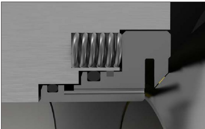
Figure-3 - Metal to metal hoop design*
