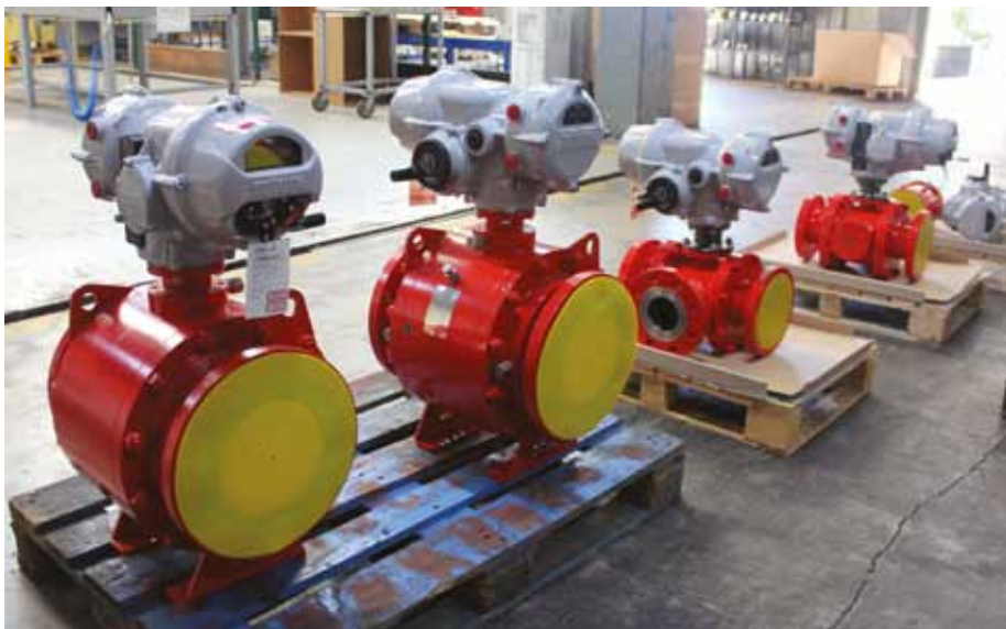
Figure 4. Automated ball valves with smart technology for real-time monitoring and control
